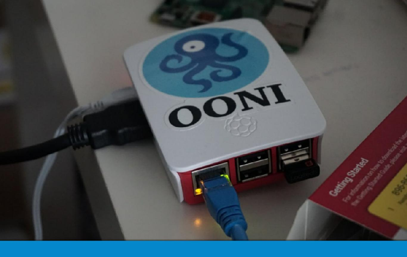
ooniprobe on RaspberryPi
